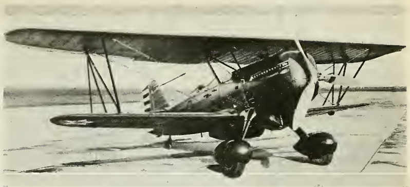
The Conqueror-powered Army Air Corps' P6E Curtiss Hawk, with liquid-cooled engine
